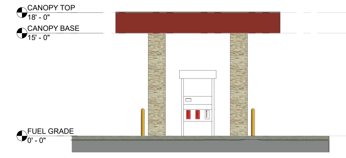
D1 CAR CANOPY - NORTH ELEVATION AS201 1/8" = 1'-0" REF'D : AS101
